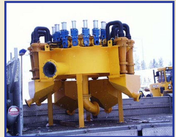
Multi Cyclones Unit
